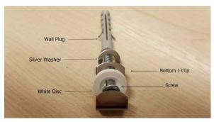
Fix non-adjustable (smaller) brackets on bottom line and adjustable (larger) on top. For 6mm Polished or arissed edge mirrors but the silver washer behind the J Clip. For 4mm mirrors and bevelled edge mirrors but the silver washer behind the white disc. Always ensure you use the correct wall plug for your wall. We supply wall plugs suitable for a brick wall. If in doubt, ask your local
