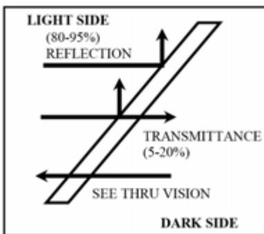
“Acrylic TV Mirror” is a semi-transparent film of aluminium deposited on an acrylic or polycarbonate substrate. This allows a percentage of incident light to pass through while reflecting the remainder. From the illuminated side, it is a mirror whilst the tv or monitor is off, however when switched on the image comes through the TV Mirror.
